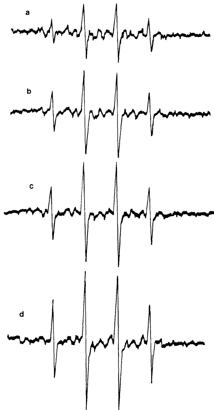
FIGURE 3 Spin-trapping spectra coupled with ESR. Spectra obtained following the incubation of chondrocytes ( 10^6/\text{ml} ) with menadione ( 10^{-2} M) in the presence of DMPO ( 10^{-1} M), DETAPAC ( 10^{-2} M) in phosphate buffered saline. Time of incubation was (a) 5 mn, (b) 15 mn, (c) 30 mn, (d) 60 mn. Microwave power was 10 mW, the modulation frequency was 100 KHz with an amplitude of 1.0 G. The receiver gain was 10^6 .
